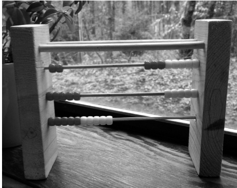
An Arbor-style rekenrek can be easily built with wood scraps, small dowels, plastic beads, a hand drill, and wood glue. Two larger-gauge dowels at the top provide stability.
